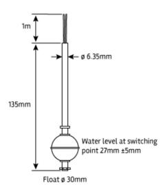
The 60 series is a small, vertically mounted liquid level sensor designed for high temperature/high
